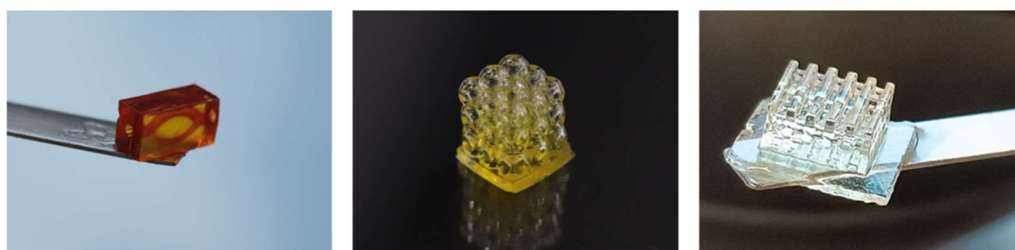
Figure 2: Left: Blood vessel structure with hollow channels perfused with a dye, Middle: Egg-shell structure and right: porous scaffold printed with BIORES INX ®
