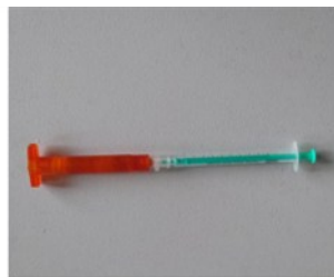
Connect EASYGEL INX cartridge to a syringe via a female luer-to-luer adapter.
