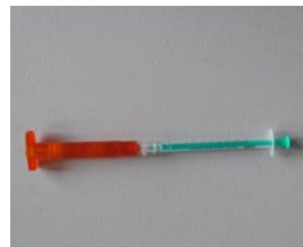
Inject cell-laden EASYGEL INX back into the cartridge via a luer-to-luer adapter.
