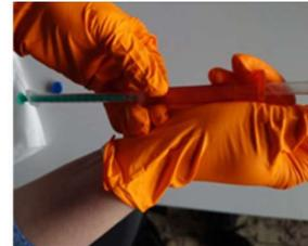
Inject the desired amount of GEL-MA INX into the syringe.
