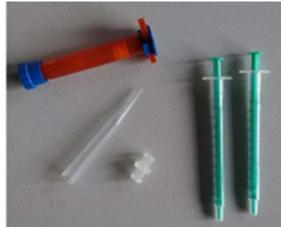
Preheat GEL-MA INX cartridge at 37 °C.
