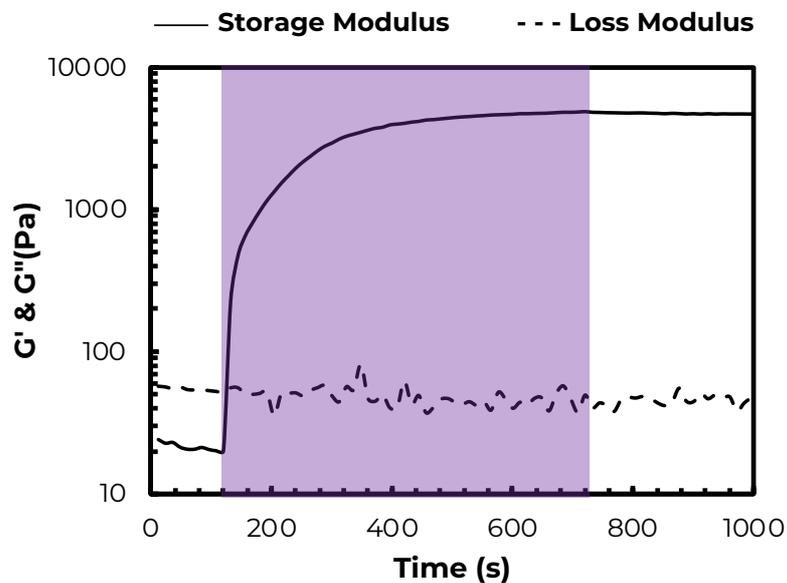
Figure 1: Storage and loss moduli of HYDROBIO INX<sup>®</sup> X100 during UV crosslinking with a UV photo-initiator
