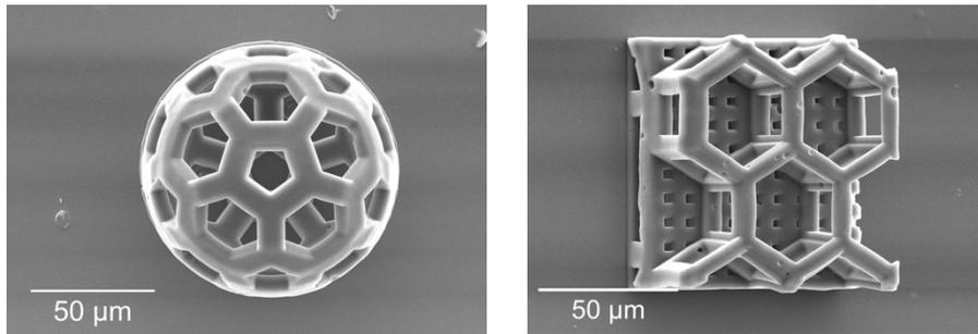
Figure 1: Scanning electron microscope images of the structures printed using HYDROTECH INX<sup>®</sup> X100 via multi-photon lithography
