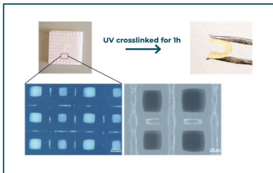
Figure 2: Photographs and optical microscopy images of a scaffold printed using a 27 G conical nozzle.
