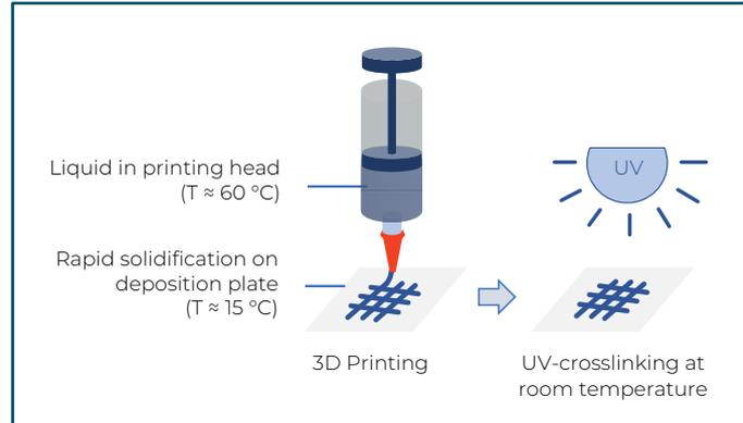
Figure 1: Schematic representation for the printing of SOLID INX<sup>®</sup>
