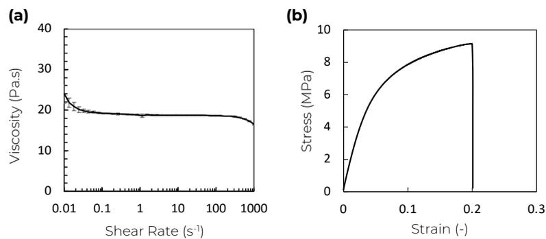
Figure 3: (a) Flow curve of molten SOLID INX<sup>®</sup> X100 as determined via rotational rheology tests at 60 °C, (b) Stress-strain curve of SOLID INX<sup>®</sup> X100.
